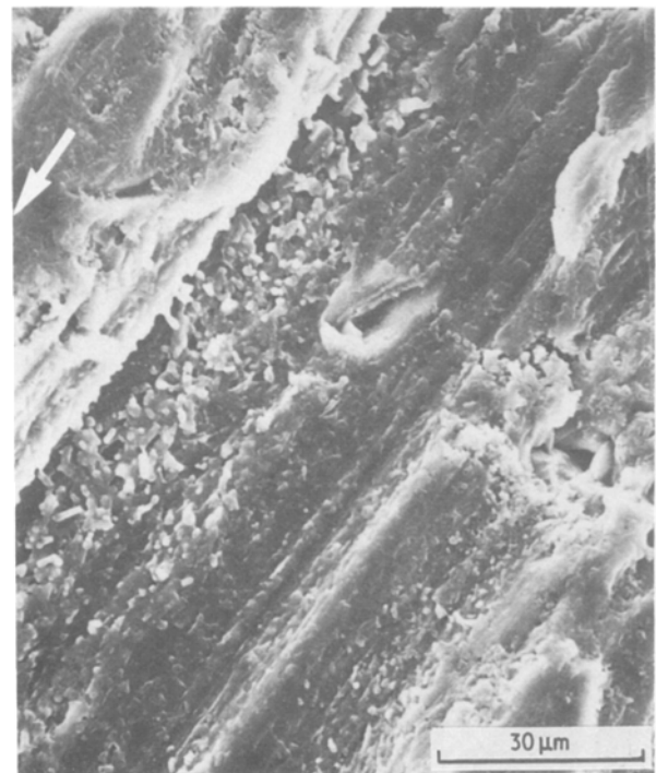
Figure 3 Higher magnification of Fig. 2b indicating abrasive particle embedded in the composite.
